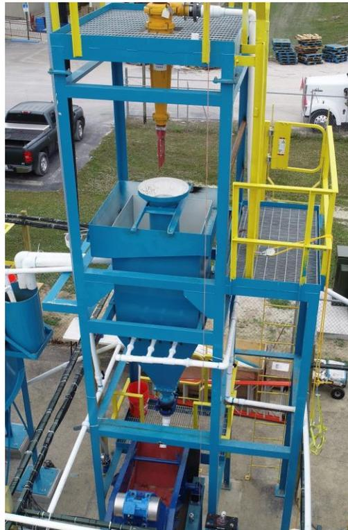
**Figure 13-6 Thickener and Decanter Centrifuge**
