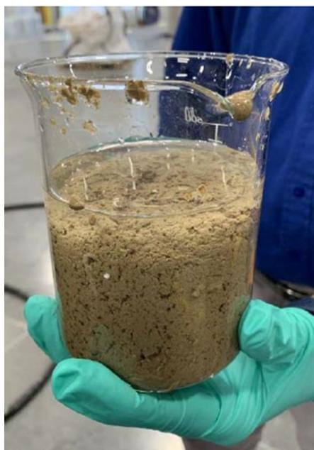
Key variables included pool depth, differential speed, polymer dosage, G-force, and feed rate. This test demonstrated that under optimized conditions, a cake dryness of 55 to 60 wt% solids could be achieved further confirming previous pilot results (Section 13.2.1.1). The machine performance during the pilot testing was used for key scale-up parameters.
