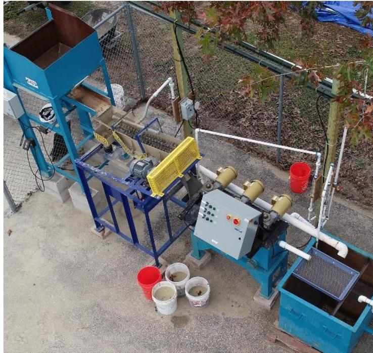
**Figure 13-5 Primary Cyclone, Hydraulic Classifier and Dewatering Screen**
