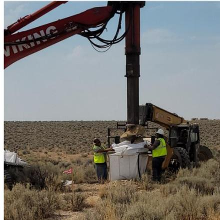
Observed auger sampling of claystone/ash material.
