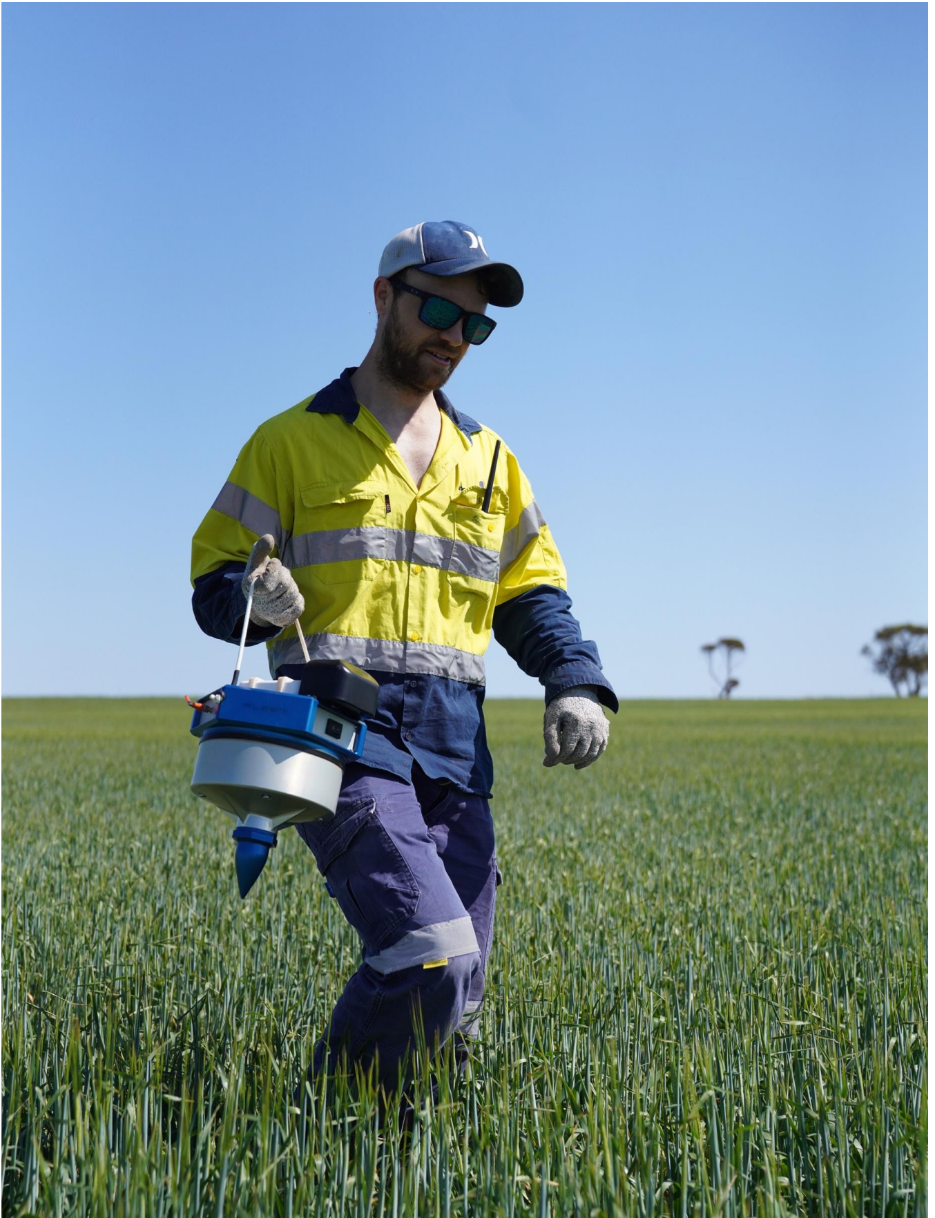
▲ Photo 5: Deployment of Exosphere by Fleet® geodes for ANT Surveys, at Alford East Project
