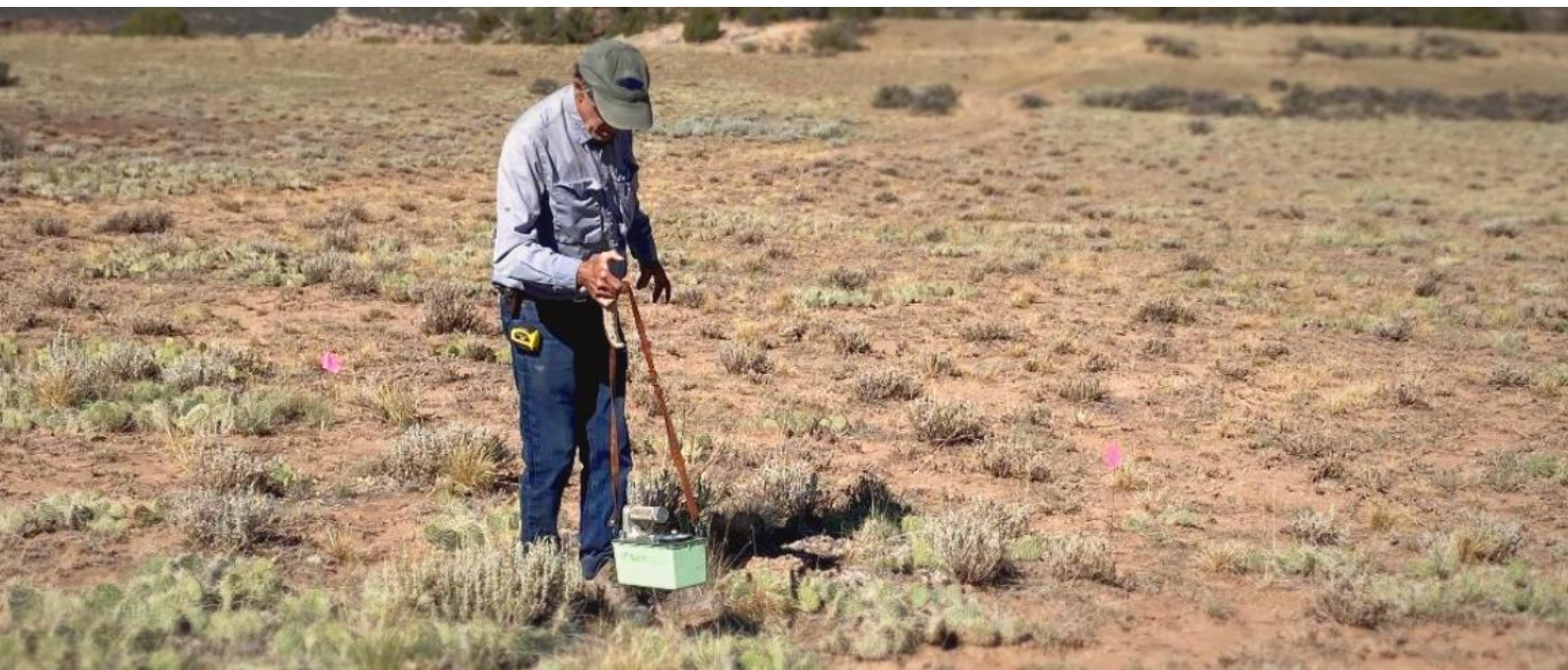
▼ Photo 4: Collecting background Scintometer readings over proposed drill pads at the Wedding Bell Project (2024)
