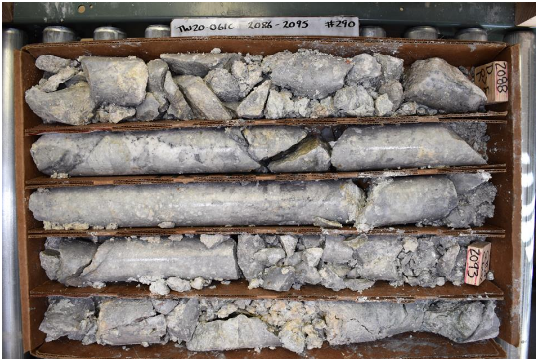
Figure 7-5 Victor Vein Drill Hole Interval 635.8 to 638.6 Metres Hole number TW20-061C; assay range: 18.23-205.5g Ag/t, 0.15-1.77g Au/t
