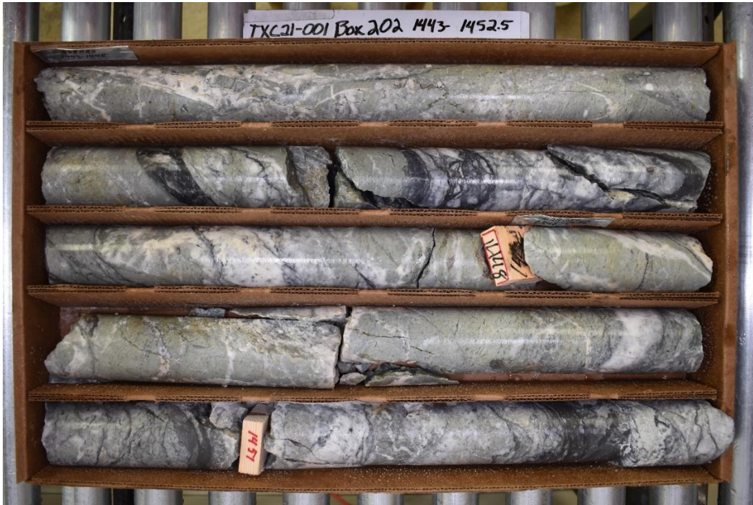
Figure 7-4 Denver Vein Drill Hole Interval 440.0 to 442.6 Metres Hole number TXC21-001; assay range: 86.1-220.0g Ag/t, 0.83-1.73g Au/t
