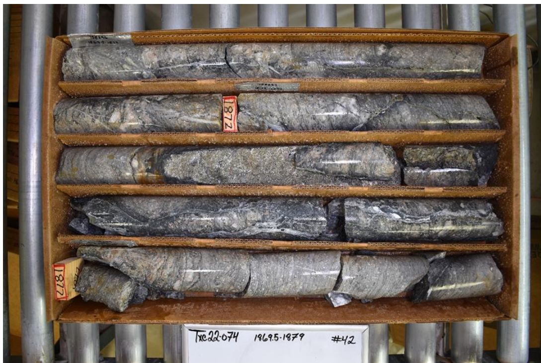
Figure 7-6 Northwest Step Out Vein Drill Hole Interval 570.6 to 572.1 Metres Hole number Txc22-074; assay range: 13.0 - 334.0g Ag/t, 0.22 - 3.78g Au/t
