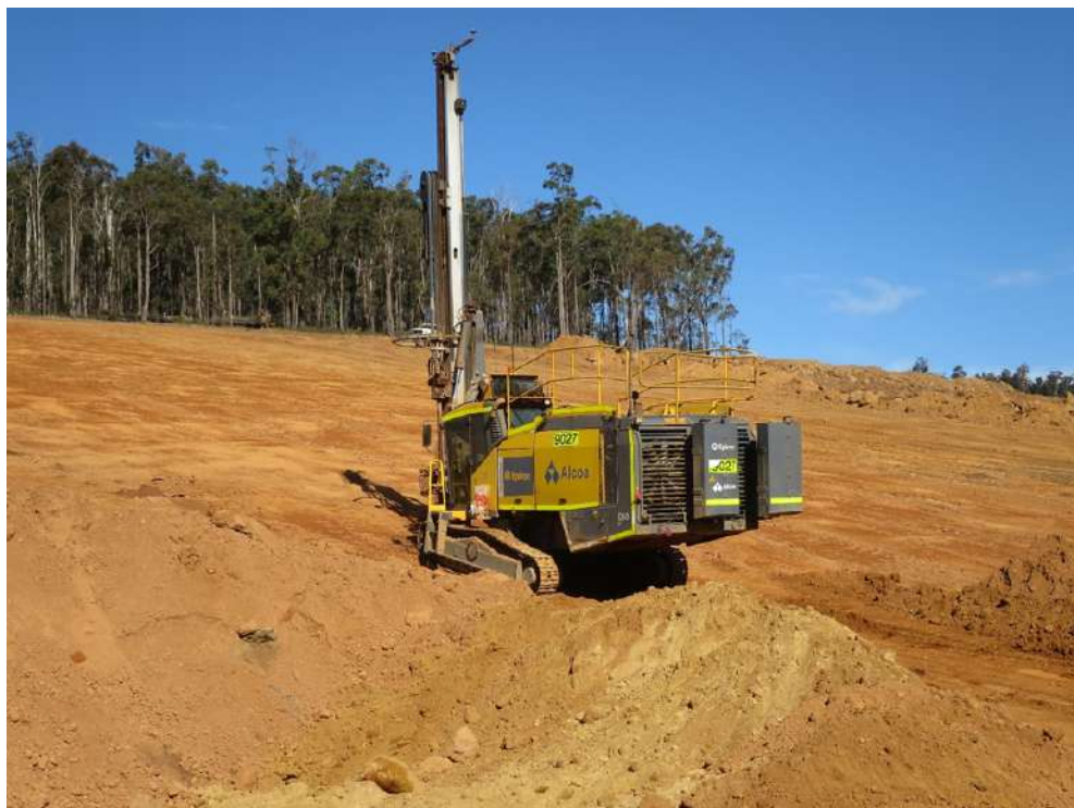
Figure 13-12: Blasthole Drill Working on Hardcap (SLR, 2021)
