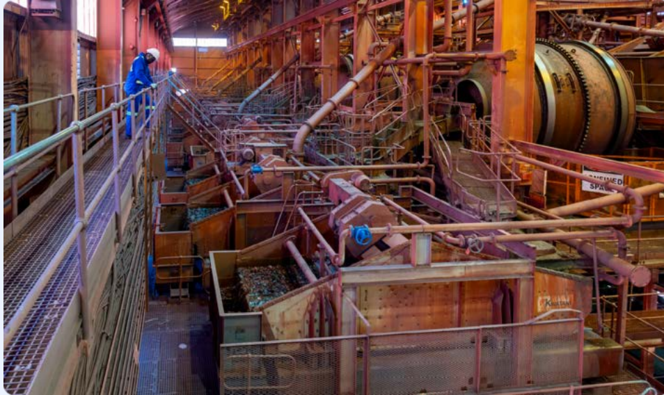
Dense media separation (DMS) processing plant at Sishen, with the current DMS drums to be upgraded as part of ultra high dense media separation (UHDMS) technology project.
