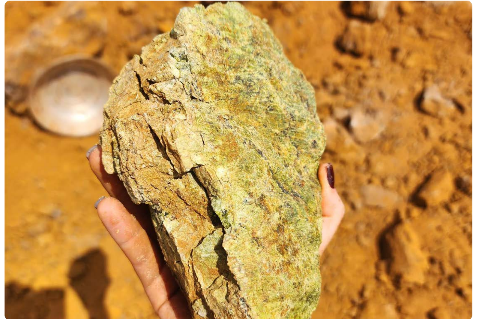
A greenish acid saprolite sample from Area 1 of the Barro Alto mine in Brazil. The sample is primarily composed of limonite, goethite and hydrated clay minerals from the smectite group.
