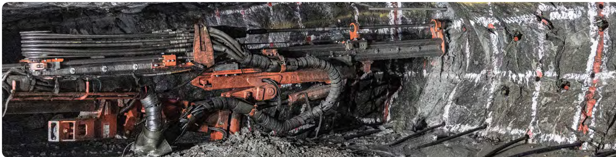
Drilling the face at an underground mining section at Unki
