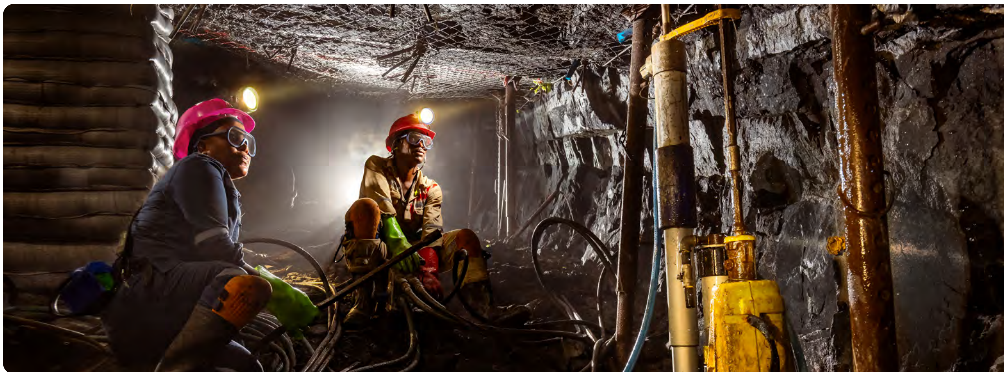
Bolting in stope with wire mesh netting at Amandelbult, Dishaba
