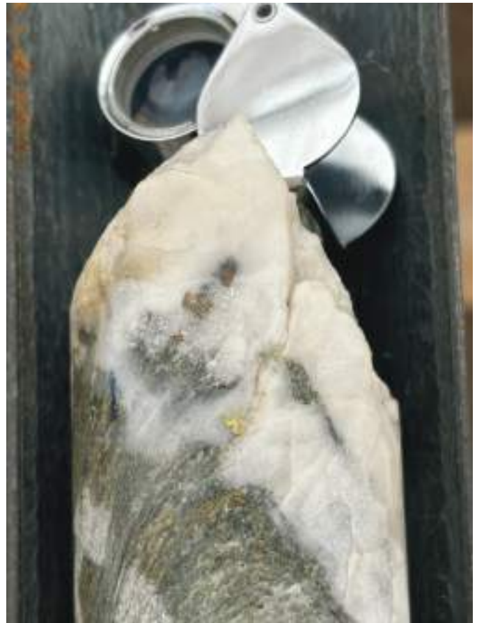
Fig. 7. Core with visible gold in quartz vein, Quesnelle Gold Quartz project (Golden Cariboo Resources Ltd.).
