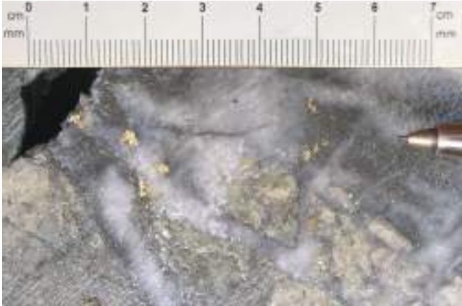
Fig. 3. Visible gold in a quartz vein at the Mineral Creek property (Karus Mining Inc.).
