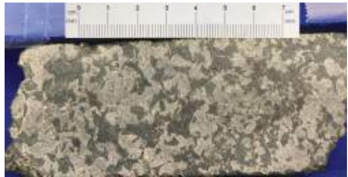
Fig. 4. Chlorite-magnetite alteration from an interval grading 1.06 g/t Au and 0.2% Cu. North Island project, Northwest Expo zone (Northisle Copper and Gold Inc.).
