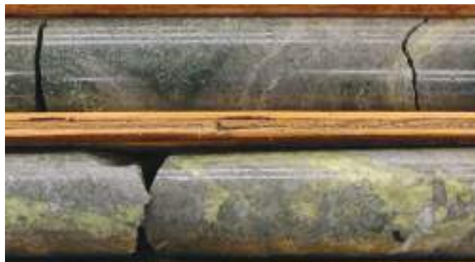
Fig. 3. Blue Sky gold zone at the Rabbit North project, RN24-055 intersection from 255.0-286.5 (31.5 m) assaying 4.15 g/t Au (Tower Resources Ltd.).
