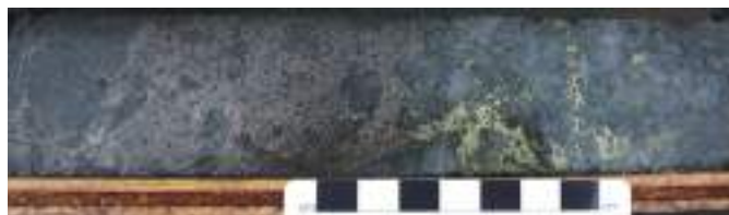
Fig. 3. Sulphide mineralization in a silicic altered zone, Bingo project (Juggernaut Exploration Ltd.).
