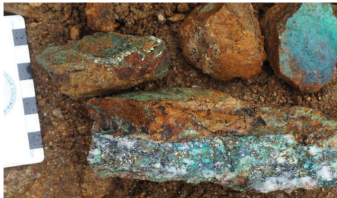
Fig. 5. Quartz vein sample with sulphides. Copper Ridge, Knauss Creek (Prospect Ridge Resources Corp.).
