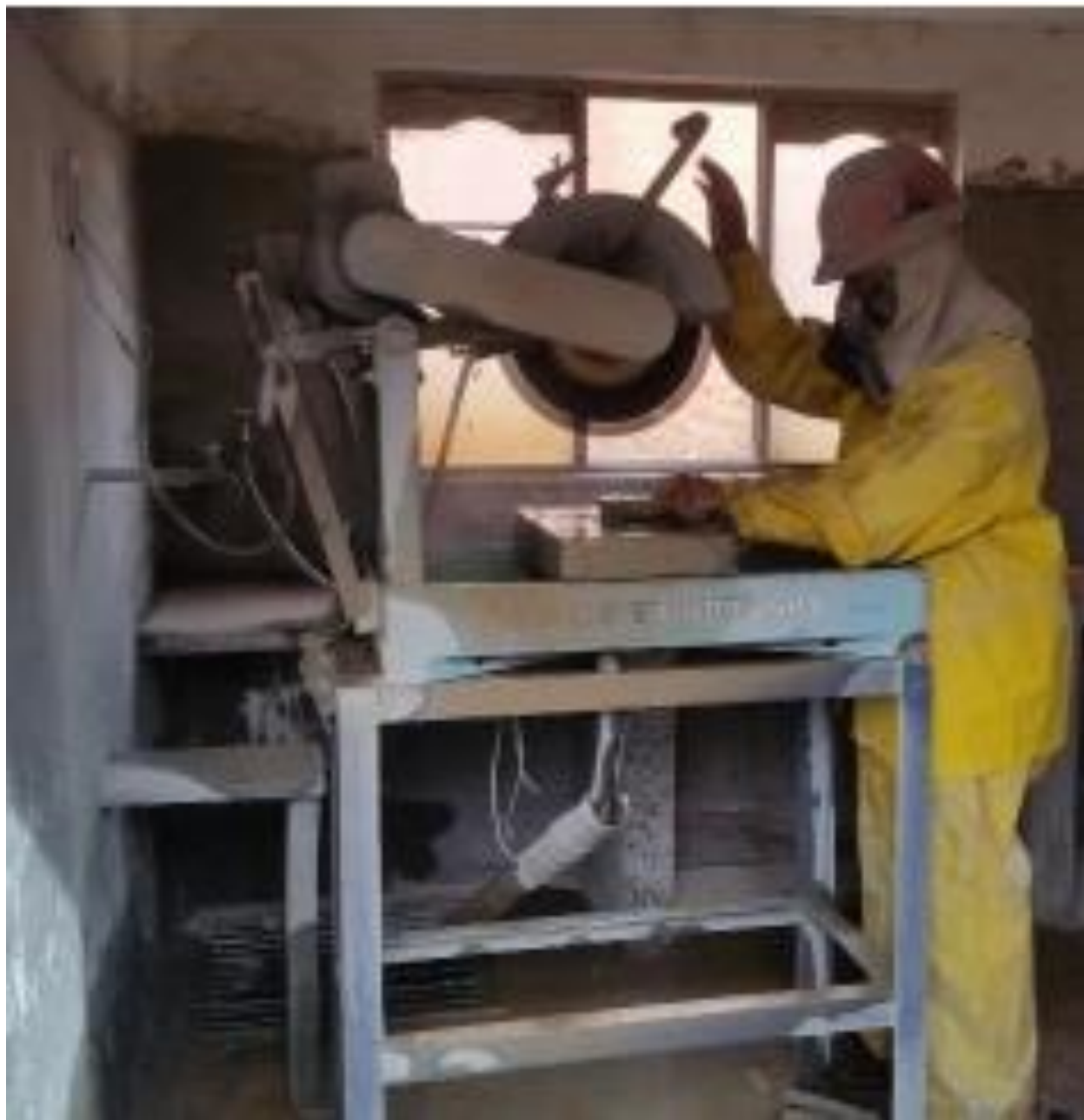
Figure 11-2: Core Splitting Facilities
