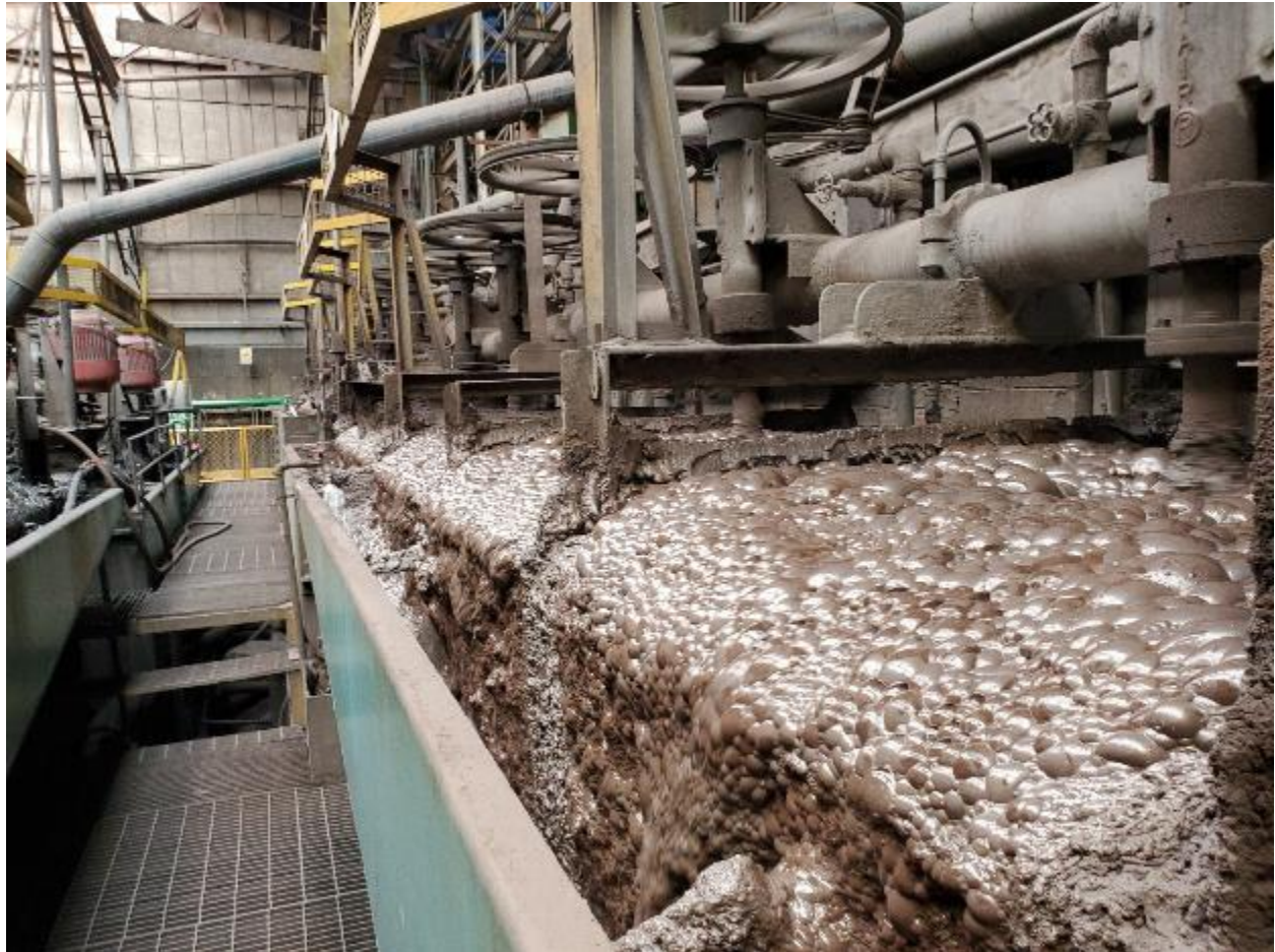
Figure 17-3: Don Diego Zinc Flotation
