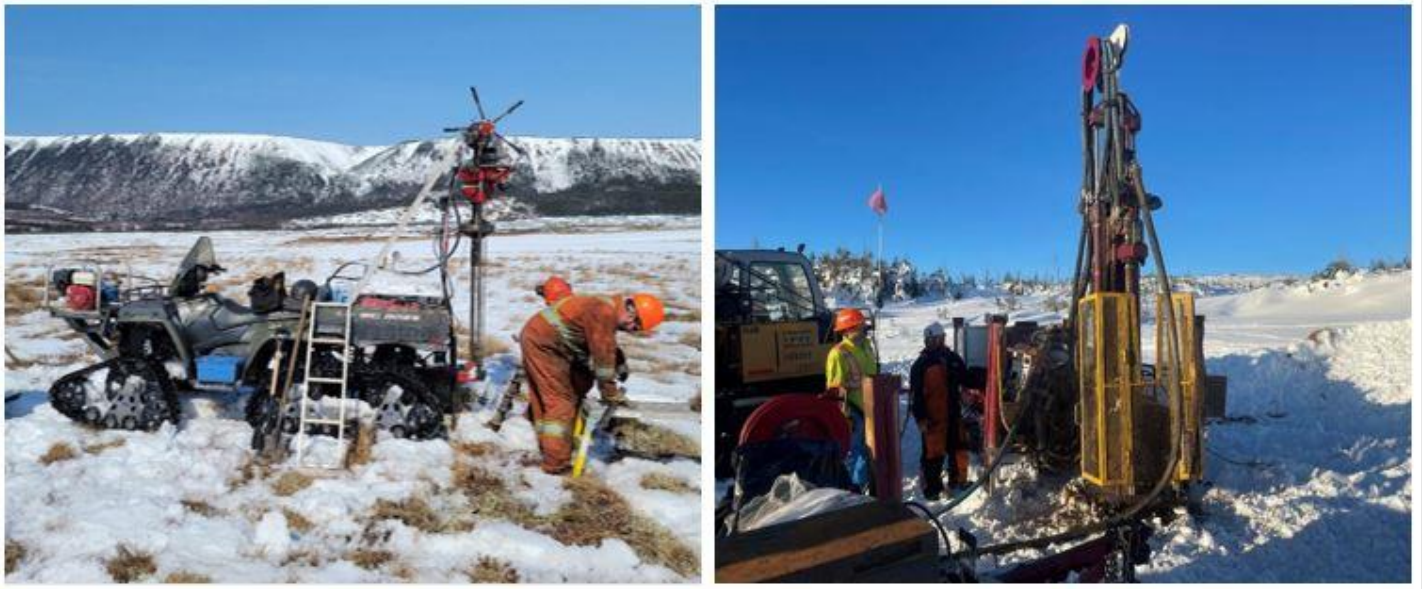
Figure 9-5: Photos showing (left) ATV-mounted Winkie drill and (right) RC drill used for top-of-bedrock and C-horizon sampling on the CR Gold Property (Source: Matador, 2023).
