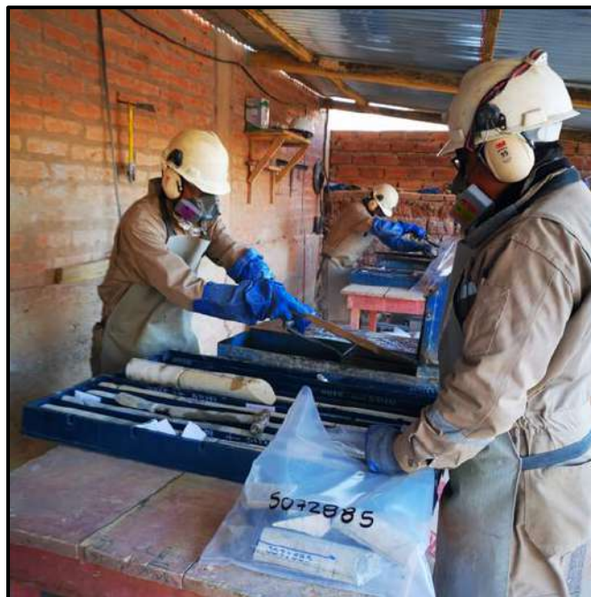
Figure 11-2 Core Cutting and Sample Bag
