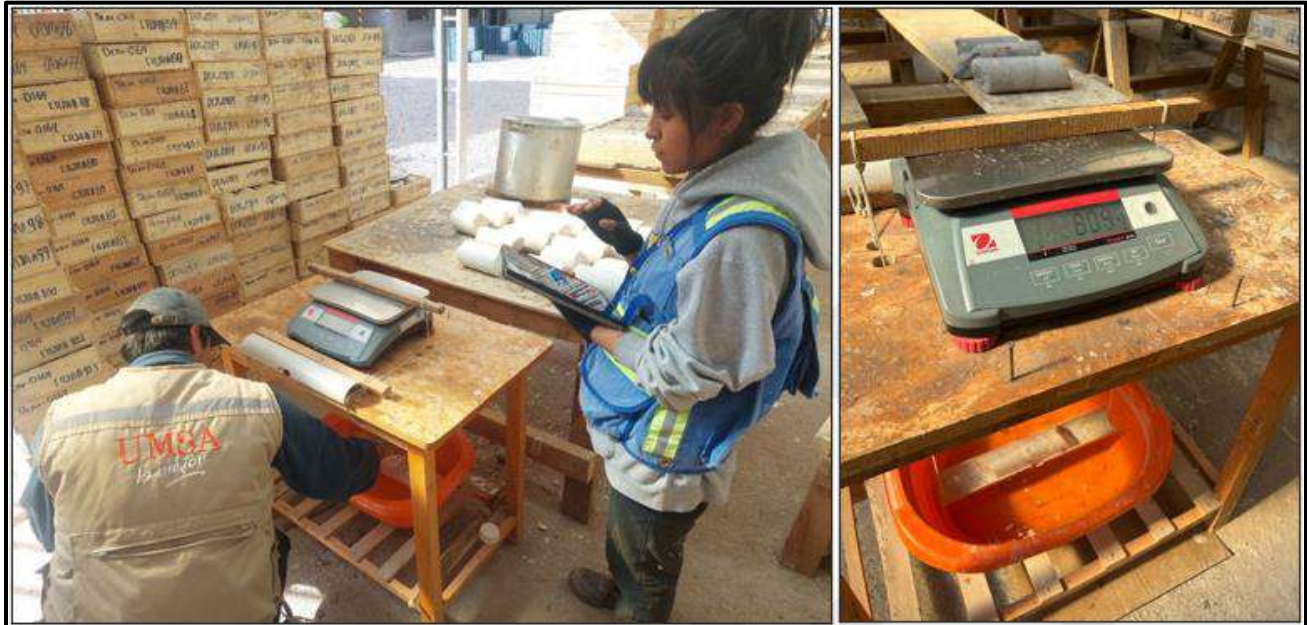
Figure 11-3 Specific Gravity Measurement
