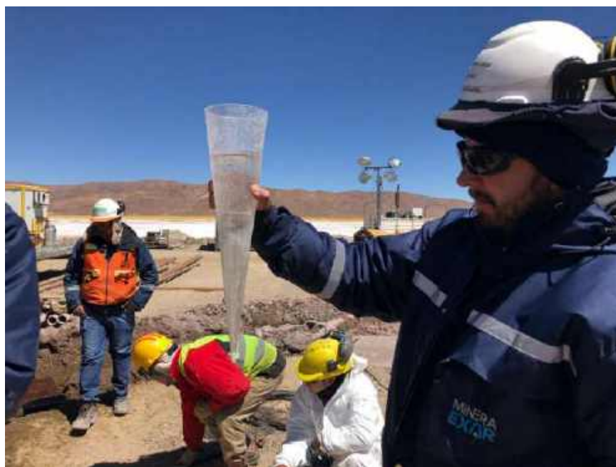
Figure 11.4 Measuring Sediment in an Imhoff Cone
