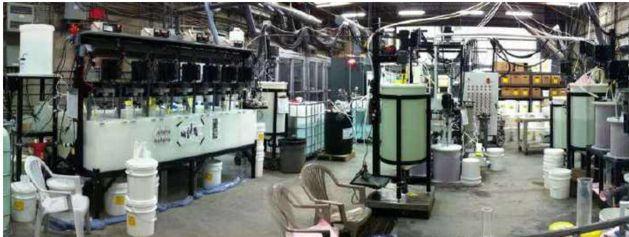
Figure 13.10 Pilot Plant (SX-Purification-Carbonation-Filtration-Washing Pulp)
