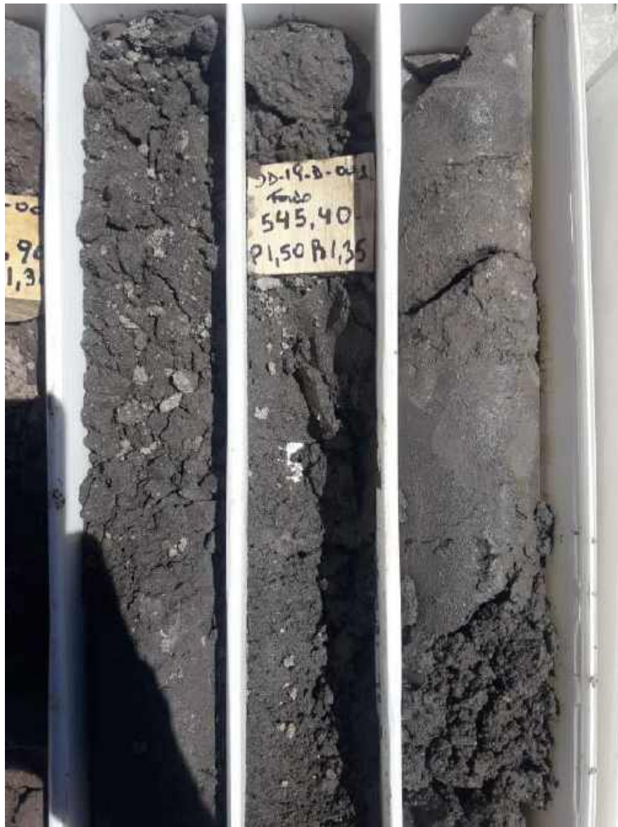
Figure 10.1 Black Sand in DD19D-001
