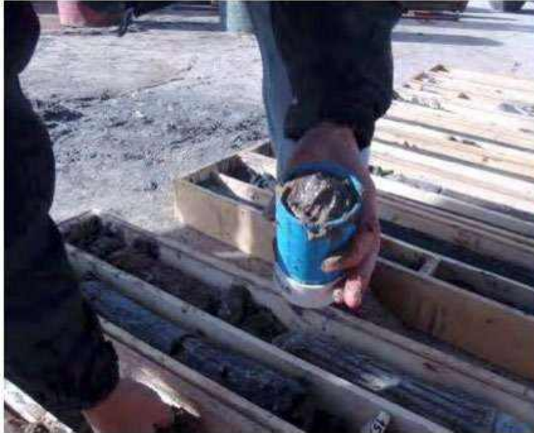
Figure 11.2 Collecting an Undisturbed Sample
