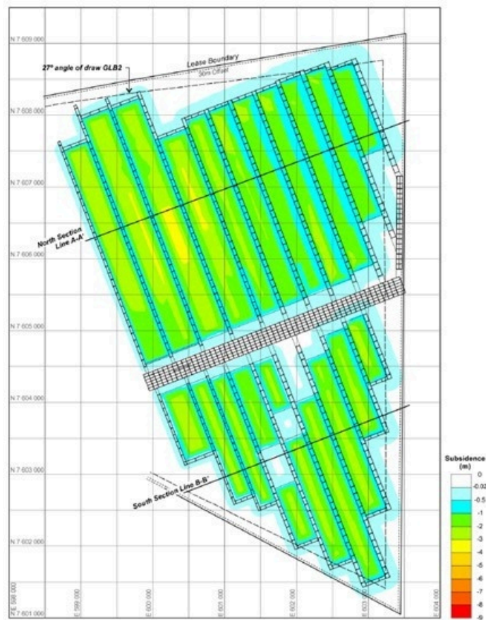
Figure 13-9. GLB2 Seam Subsidence Prediction Contours
