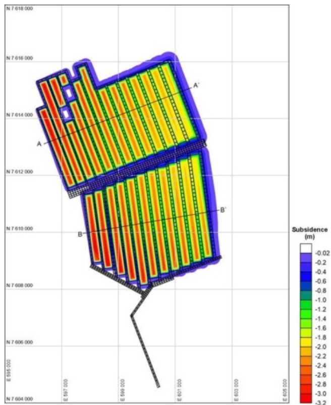
Figure 13-6. Centurion North (GM Seam) Subsidence Prediction Contours
