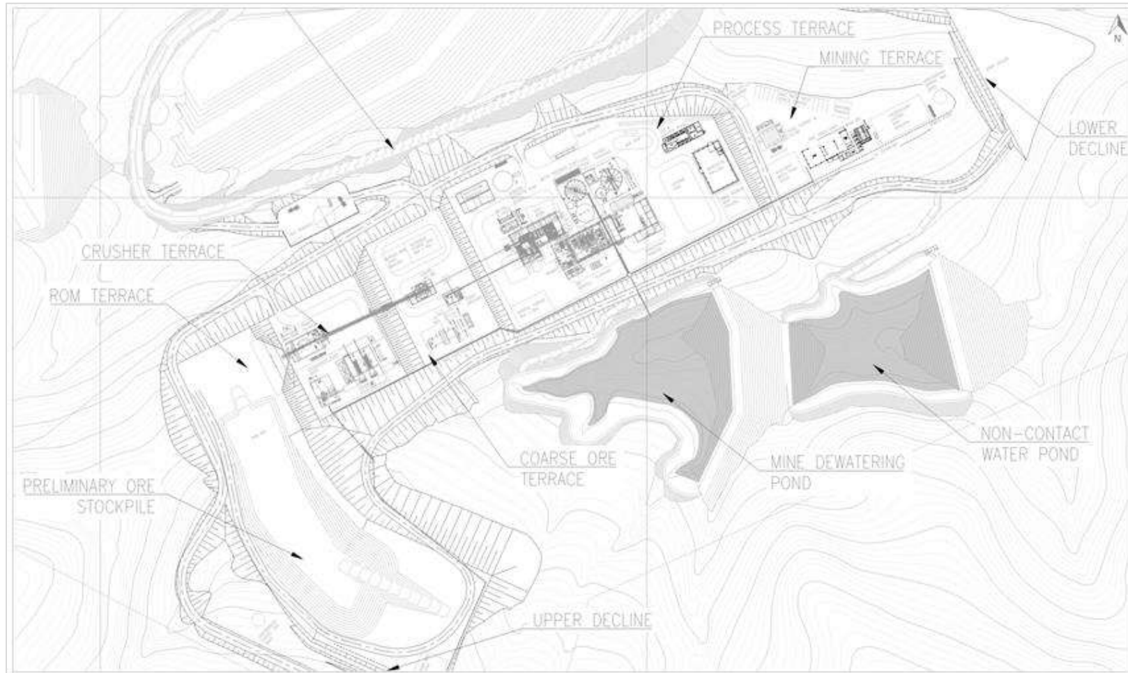
Figure 18.2 – Process Plant Layout
