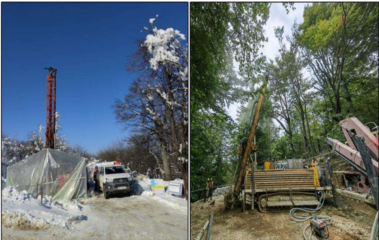
Figure 10.1 – Diamond Drill Rig (Left) and a RC Drill Rig (Right) at Čoka Rakita
