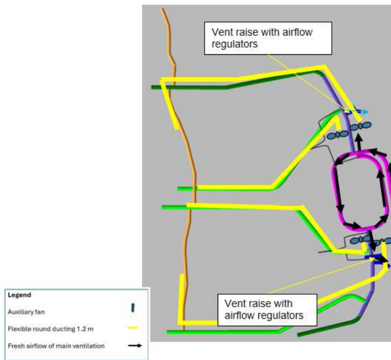
Figure 16.17 – Auxiliary Ventilation on Production Levels
