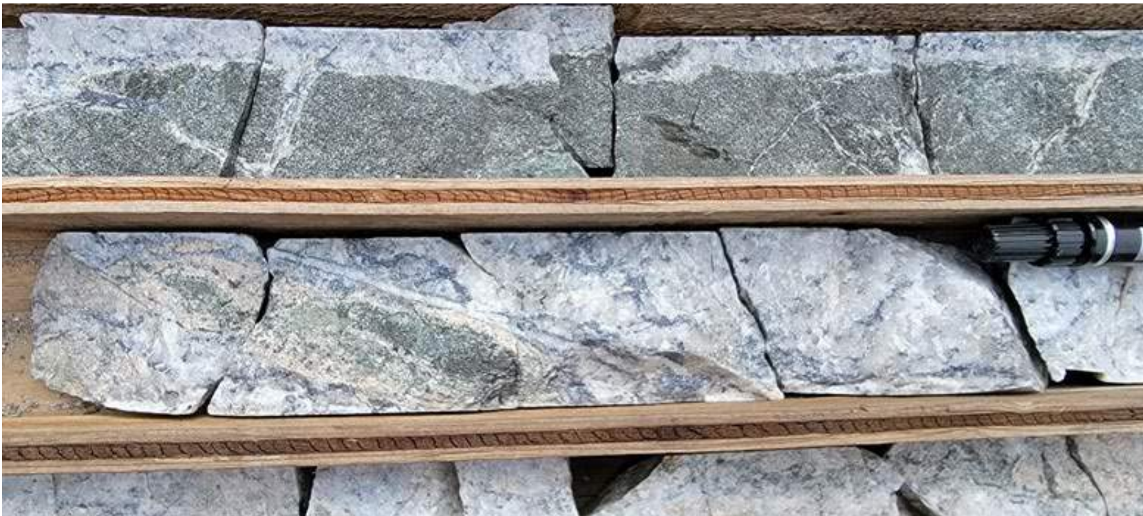
Figure 12.3. View of Some NQ Split Core (DDH 189) from Blue Pearl Era Drilling; Some Samples Were Taken to Verify Grade Source: AMPL, 2023
