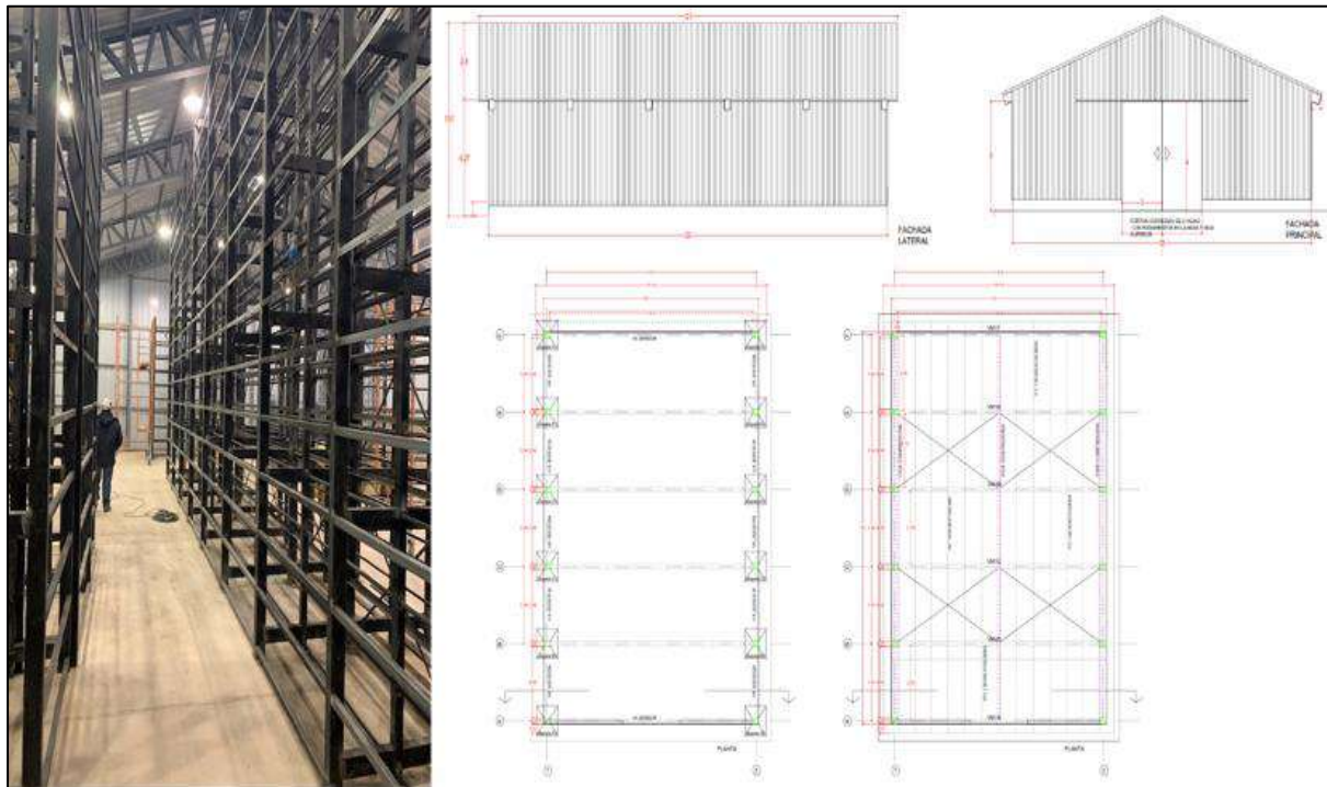
Figure 18-11: Core storage building and racks for approx. 30,000 m of cores
