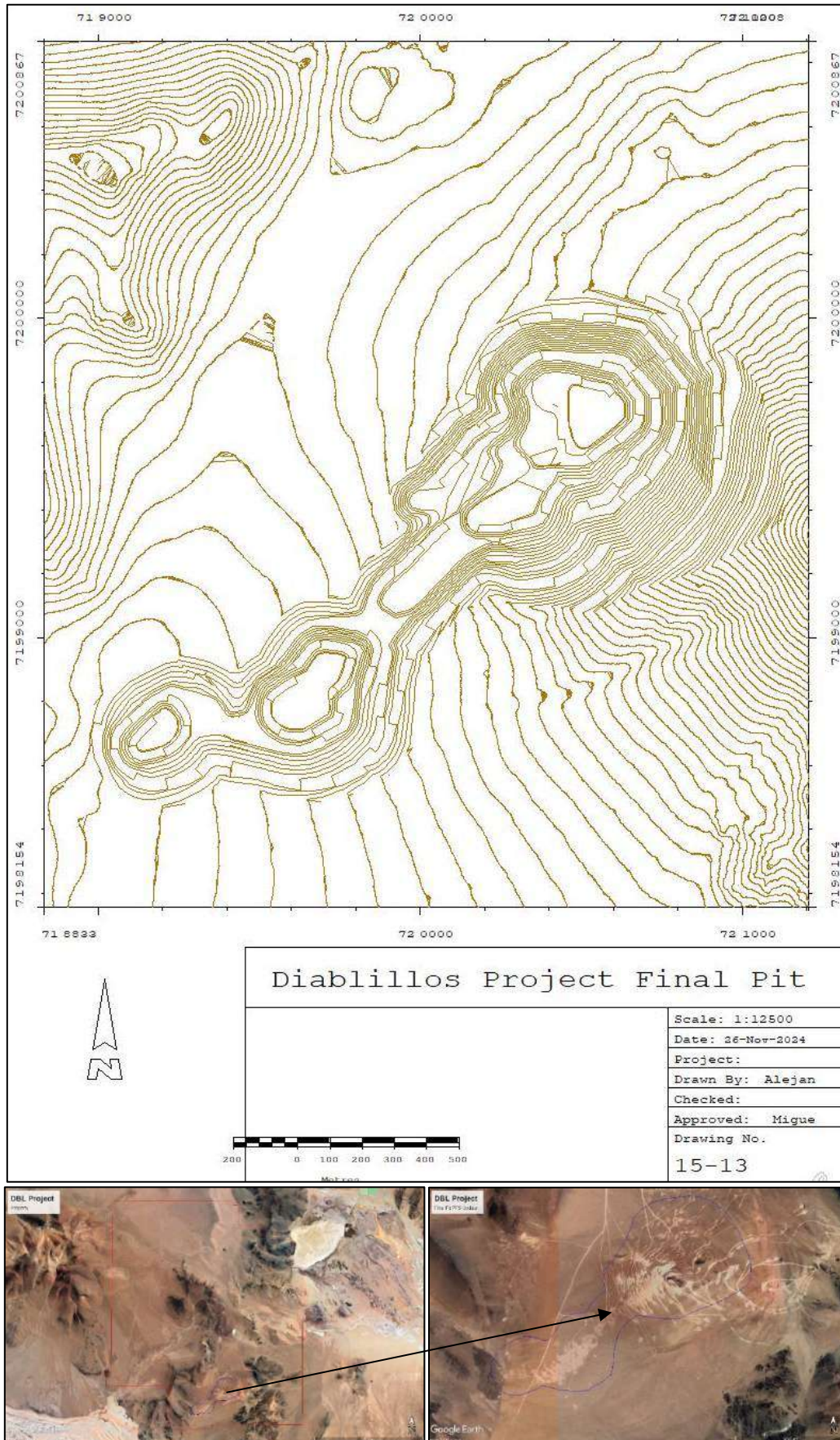
Figure 15-14: Diablillos Project Ultimate pit design
