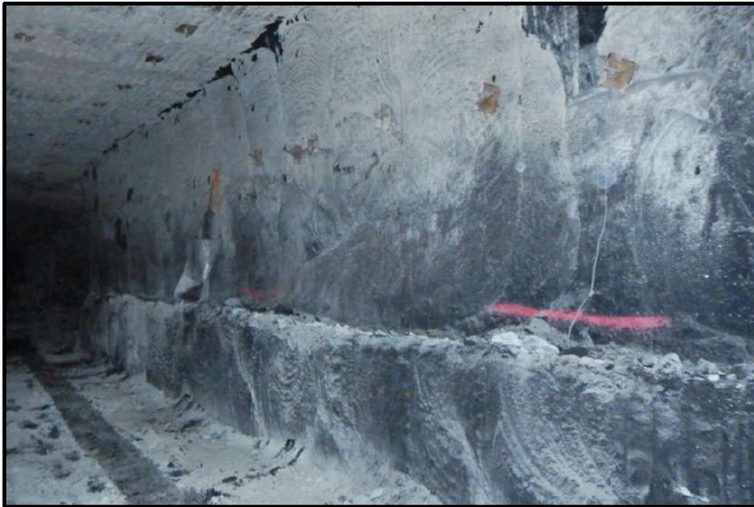
FIGURE 4-12 PAINT MARKS TO CONTROL THE THICKNESS OF FLOOR COAL MINED.
