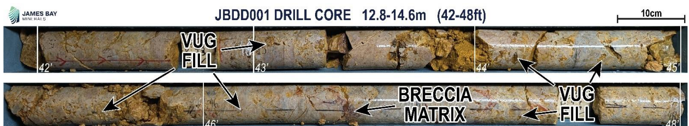
Figure 4: JBDD001 drill core at 12.8 - 14.6m (42 - 48ft) showing silica-flooded and partially brecciated vuggy chert. Highlighted are examples of iron oxide (after sulphide) vug-fill and matrix fill.
