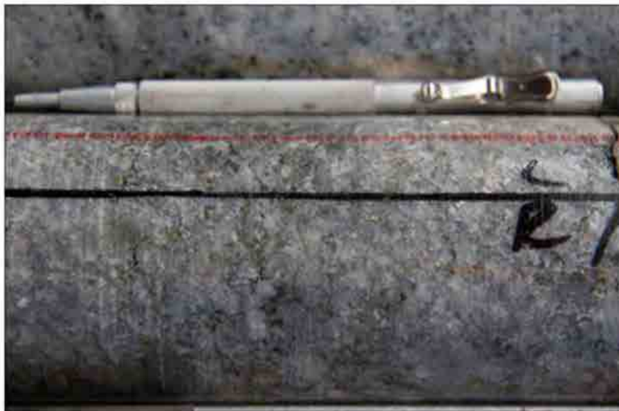
Figure 7-9 Disseminated mineralisation seen in marble within the sulphide zone
