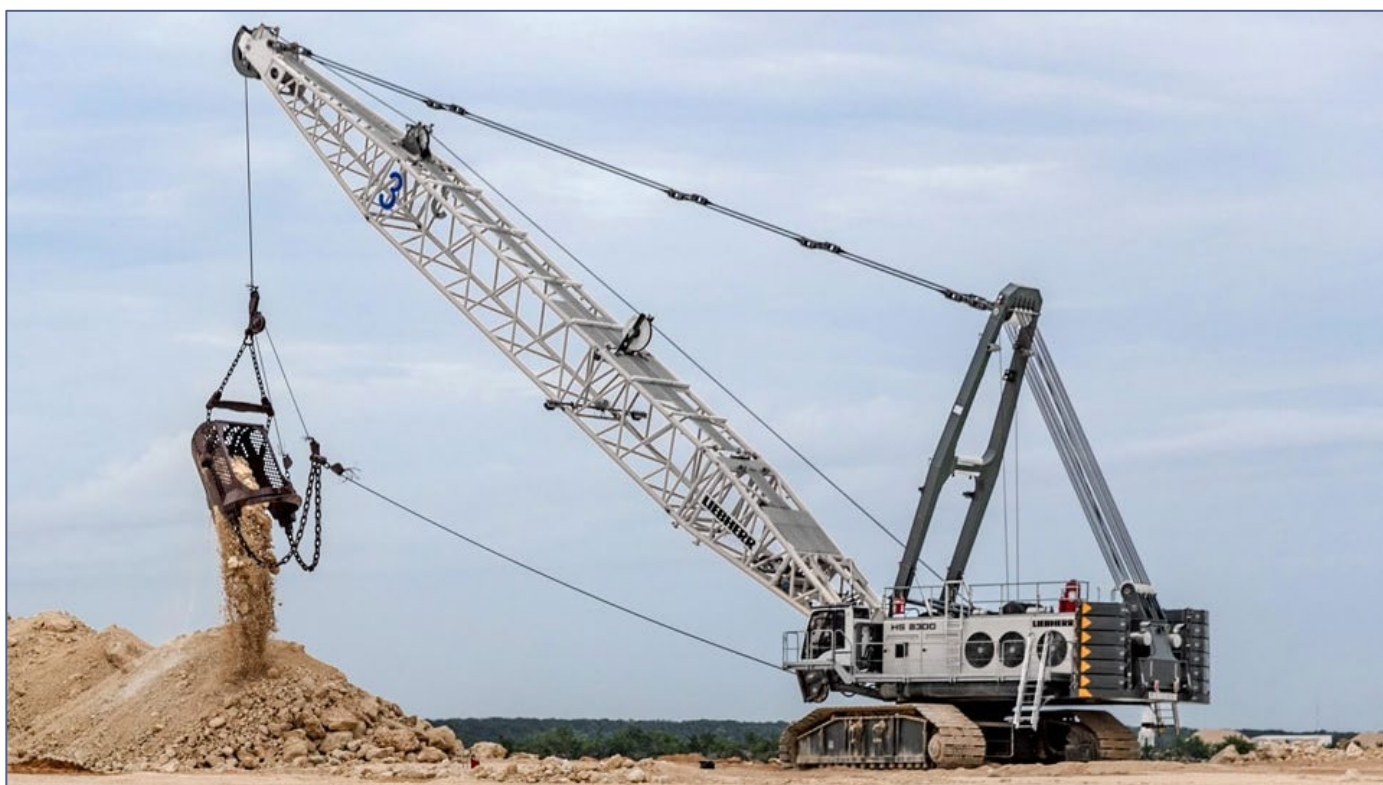
Figure 10: Example of a dragline excavator in action (Source: Liebherr Group)
