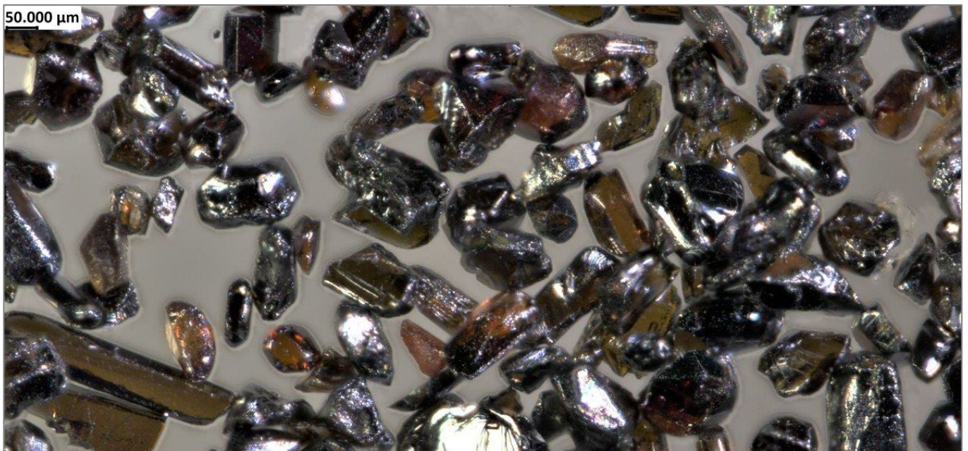
Figure 17: Photomicrograph of high-purity rutile product
