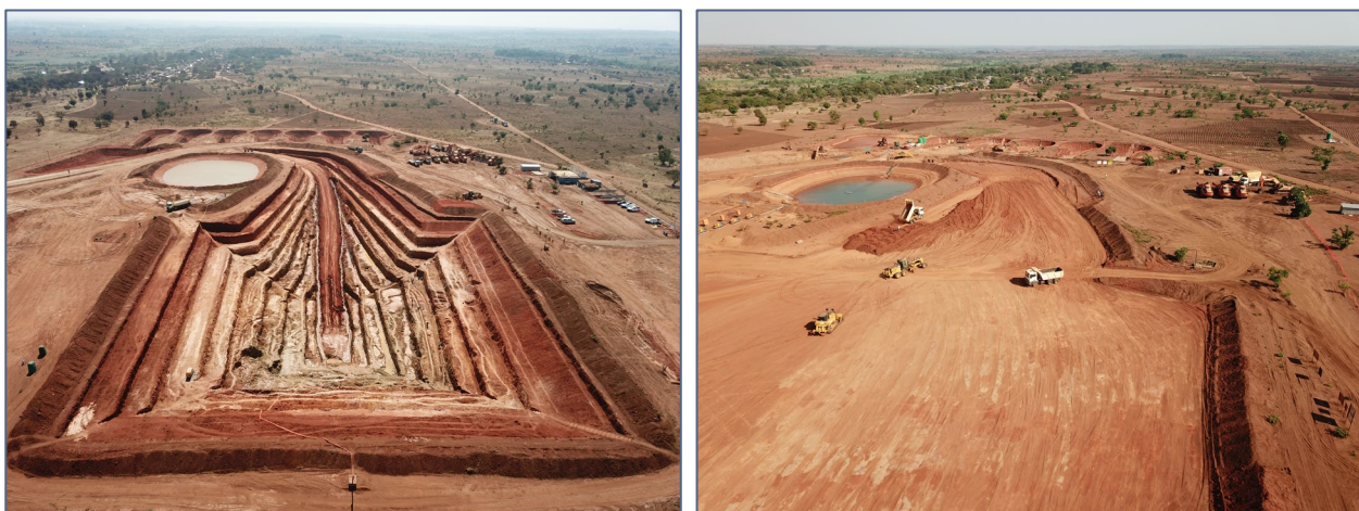
Figure 1: Pilot Phase test pit during mining trials (left) and subsequently backfilled (right)
