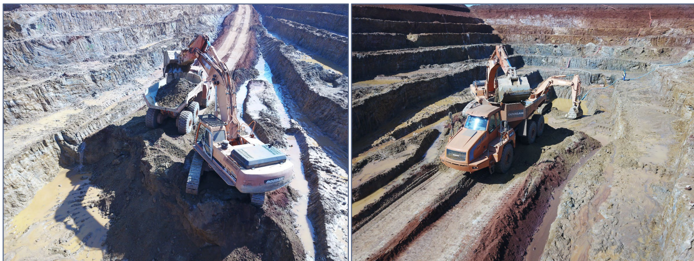
Figures 7 & 8: Simple excavator fleet mining the test pit
