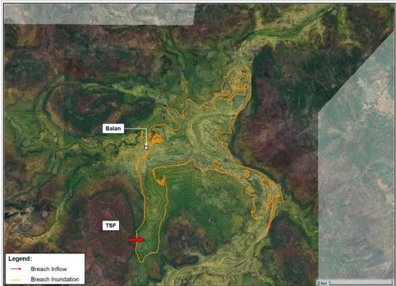
Figure 18.4 Sunny day failure scenario without conceptual mitigation measures
