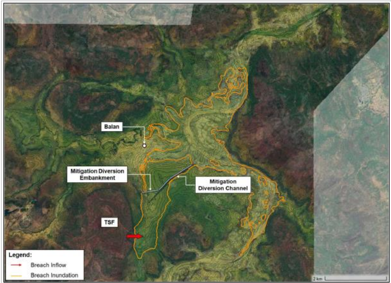
Figure 18.5 Sunny-day failure scenario with conceptual mitigation measures
