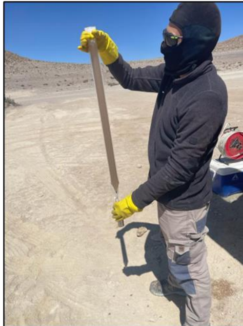
Figure 11.4 – Filled Hydrasleeve Model HS-2 Sample
