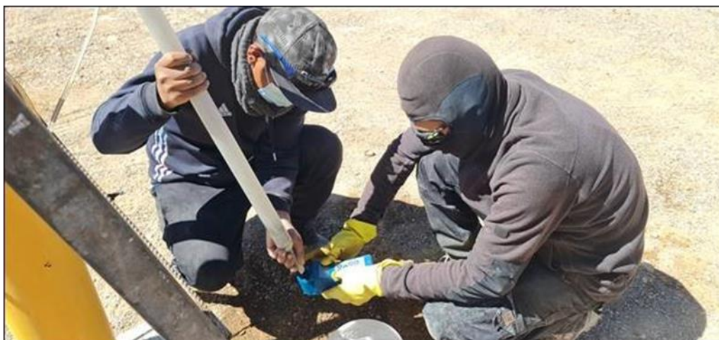
Figure 11.3 – Measuring Field Parameters During Sampling with Plastic Bailer
