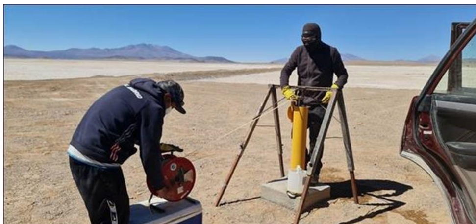
Figure 11.2 – Iron Stand Over Well Used for Sampling
