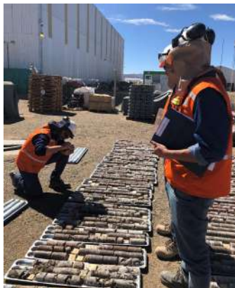
Figure 8.3 Collecting an Undisturbed Sample from Core
