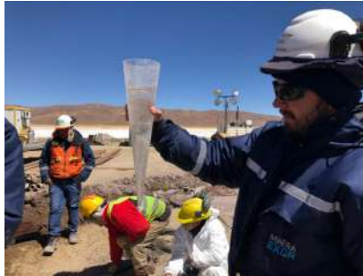
Figure 8.4 Measuring Sediment in an Imhoff Cone
