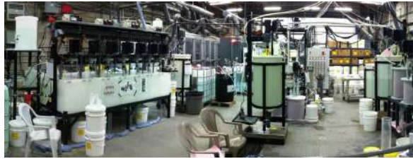
Figure 10.10 Pilot Plant (SX-Purification-Carbonation-Filtration-Washing Pulp)
