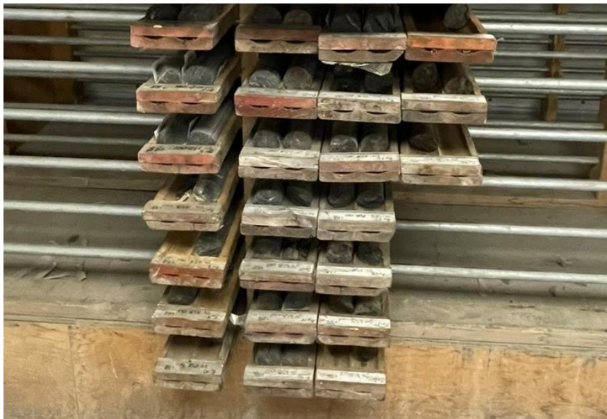
Figure 10.8 – Example of Logged and Tagged Core Ready for Cutting
