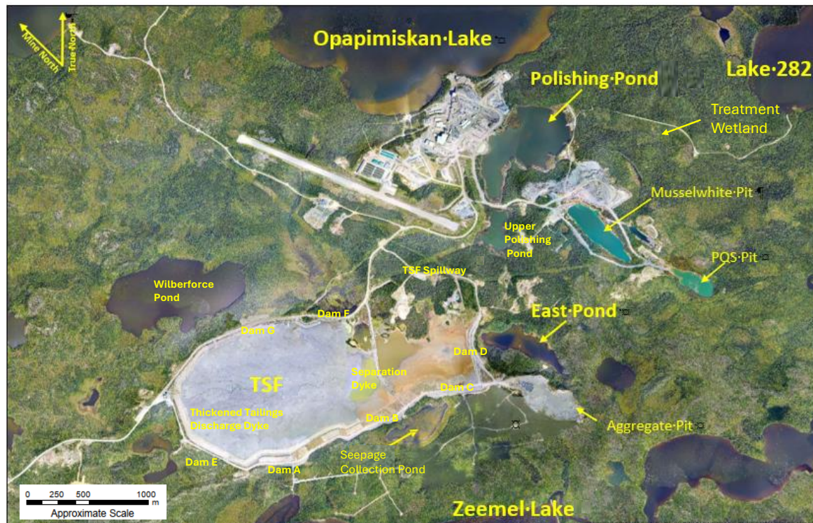
Figure 18.3 – General Arrangement of Tailings Storage Facility and Water Management
