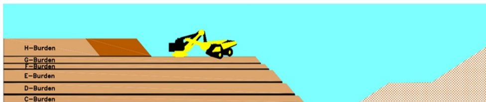
Figure 13.6 Pit Layout - Dozer operation. (Mississippi Lignite Mining Company, 2019)
