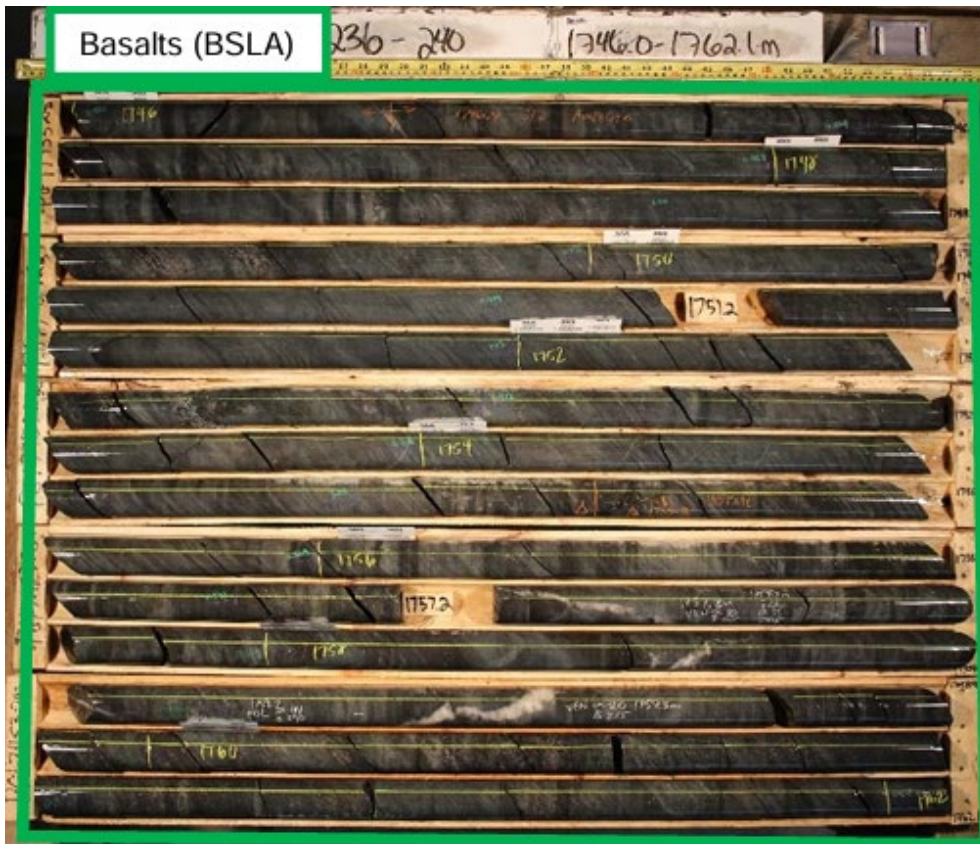
Figure 16-3: Drill core demonstrating the basalt rock mass
