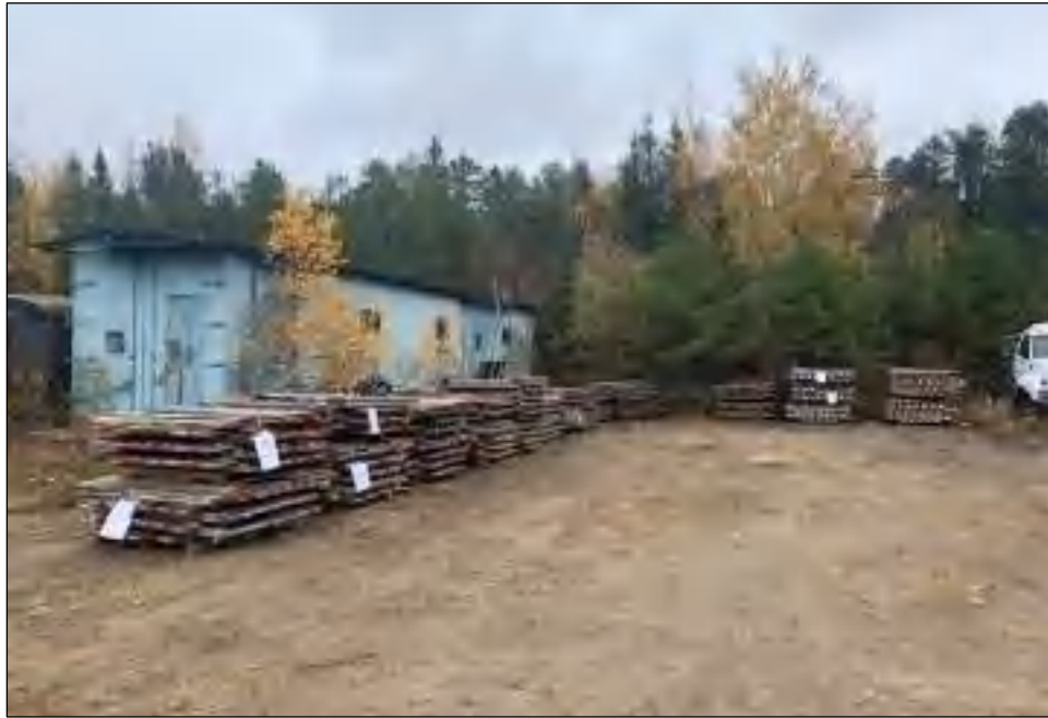
Figure 11-9: Coarse Storage Area; Core Stored in Cross-piles (Source: Nordmin, 2023)
