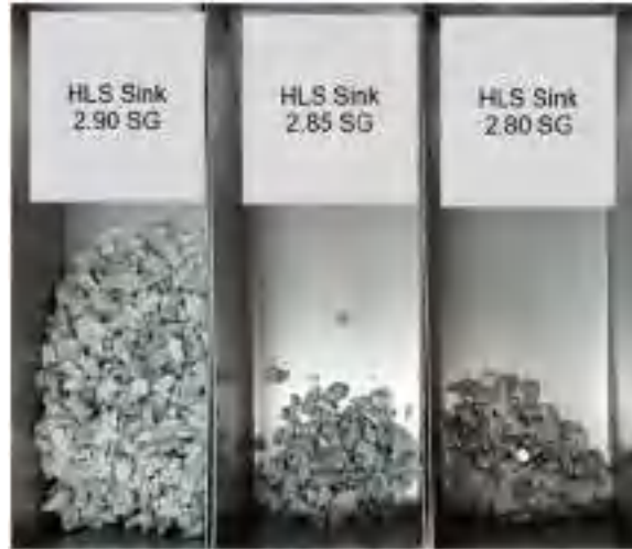
Figure 2: HLS Sink Products of 2.80, 2.85, and 2.90 SG from -12.7 mm +6.3 mm Fraction
