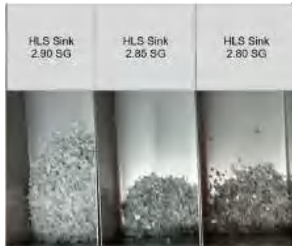
Figure 4: HLS Sink Products of 2.80, 2.85, and 2.90 SG from -6.3 mm +1 mm Fraction
