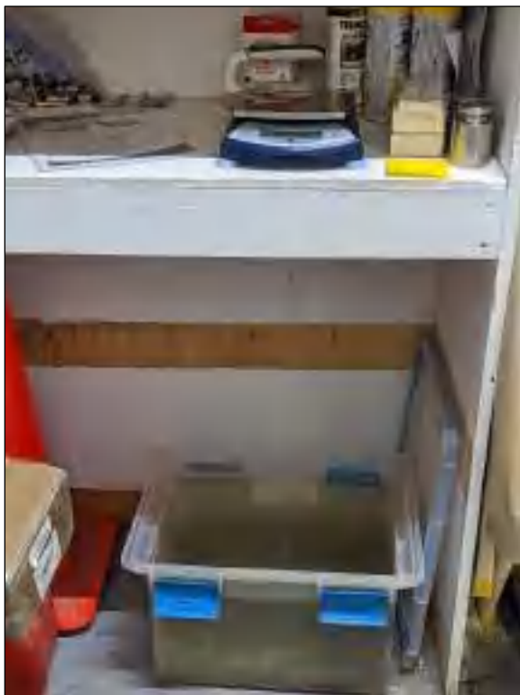
Figure 12-11: SG Weighing Station (Source: Nordmin, 2023)
