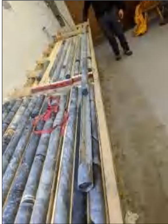
Figure 12-1: Core Shack Logging Table with Metal Bar Used for Orienting Core (Source: Nordmin, 2023)
