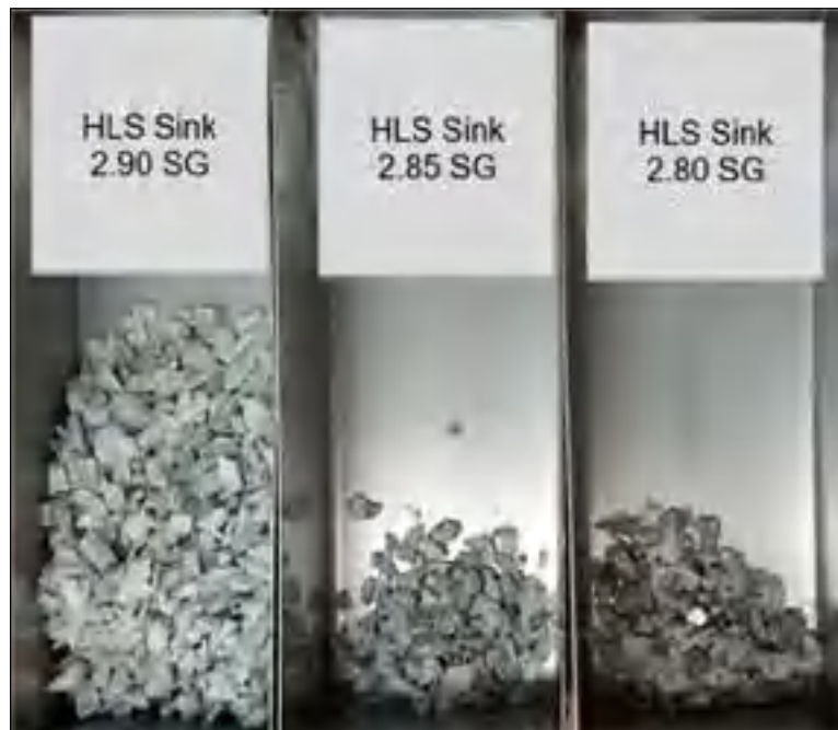
Figure 13-3: HLS Sink Products of 2.80, 2.85, and 2.90 SG from -12.7 mm +6.3 mm Fraction
