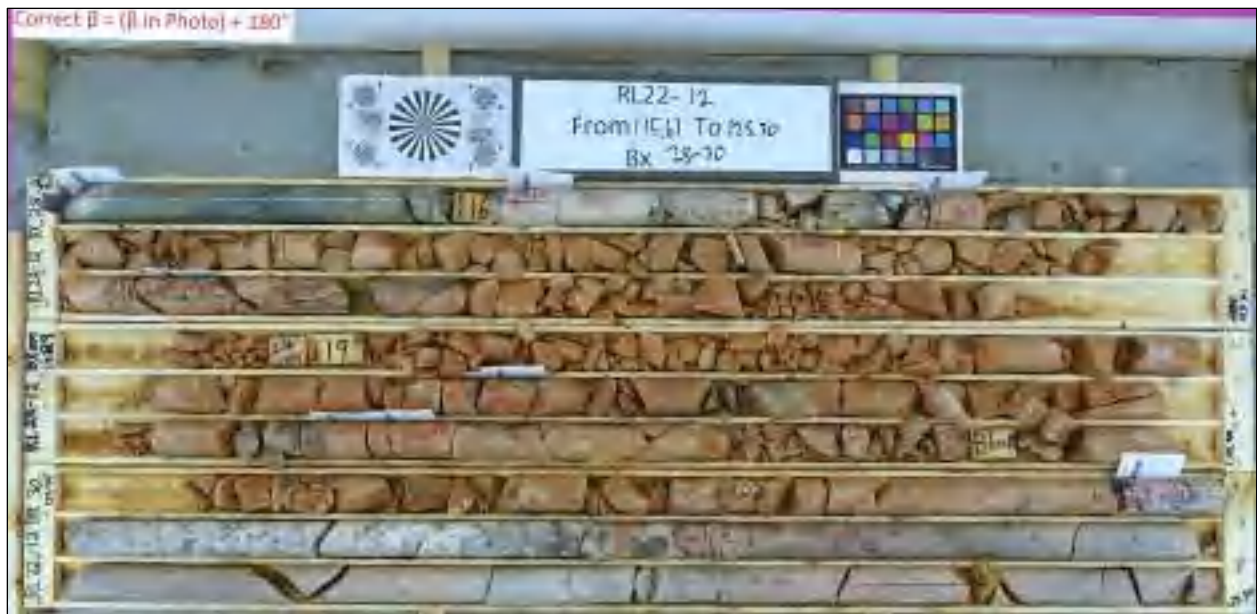
Figure 12-4: Interval of Rb Rich Microcline Mineralization within Pegmatite from RL22-12 from 115.61 m to 125.90 m (Source: Nordmin, 2023)
