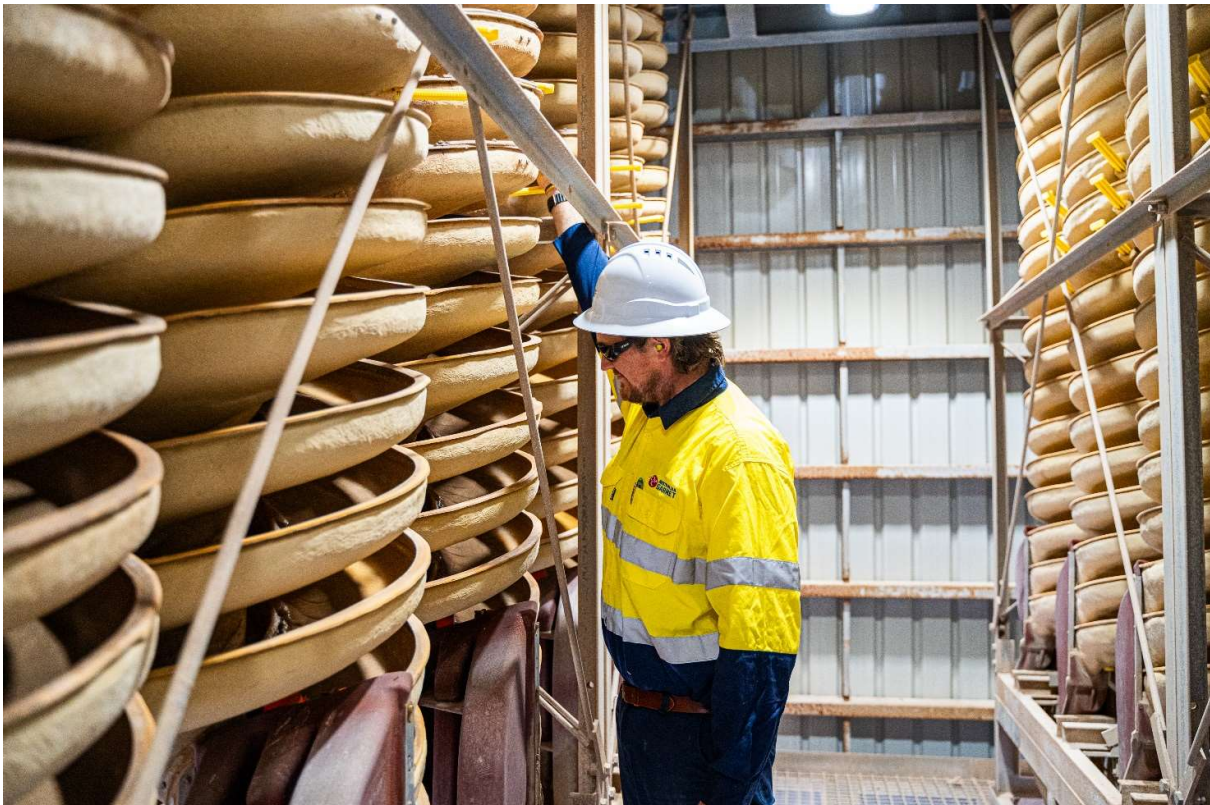
Figure 4 Wet Concentrator Plant Spirals at Lucky Bay
