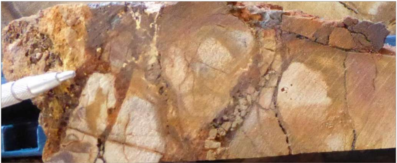
Note: DSS525001 Oxidized crackle breccia @ 65.30 m (892 g/t Ag). Source: New Pacific Metals Corp., 2019.
