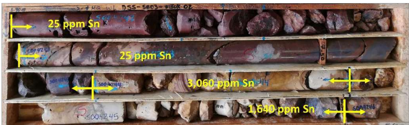
Figure 7.14 Example of tin mineralization associated contact Tarapaya with Cretaceous sandstone
