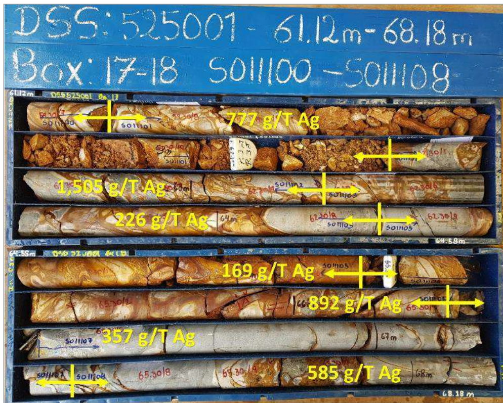
Note: Hole DSS525001 Oxidation interval (Limonite, jarosite), showing silver grades. Source: New Pacific Metals Corp., 2022.
