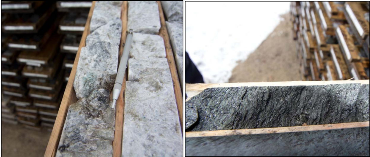
Figure 9 – Spodumene bearing pegmatite example in drill core (left) and meta-sediments host rock (right).
