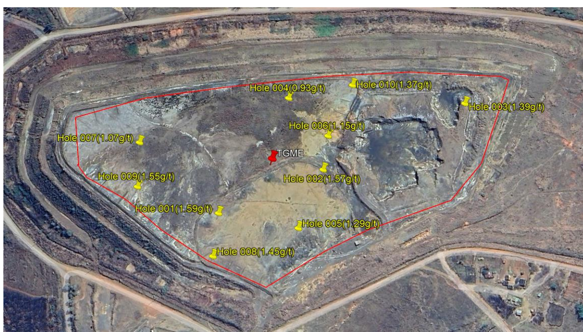
Figure 2 – Drill hole location map of the holes drilled by SGS team at the TGME Main TSF
