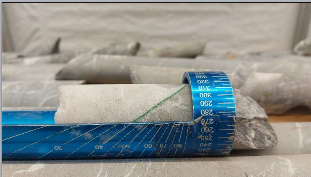
Figure 10.7: Structural Data Collection Using a Kenomneter
