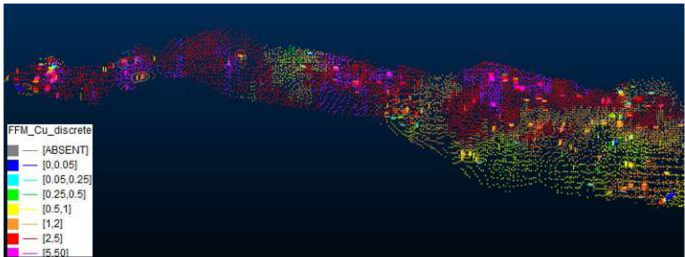
Figure 14.5: Block Copper Grades Compared to Composite Grades for Domain 1807
