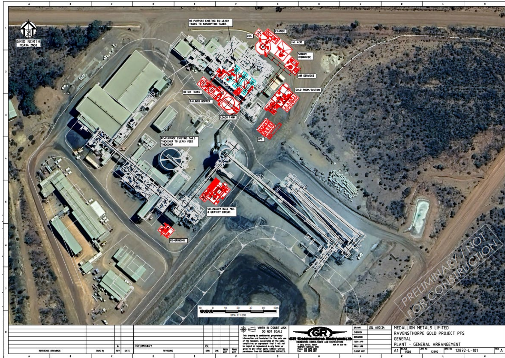
Figure 3: Cosmic Boy Process Plant with proposed modifications (red).
