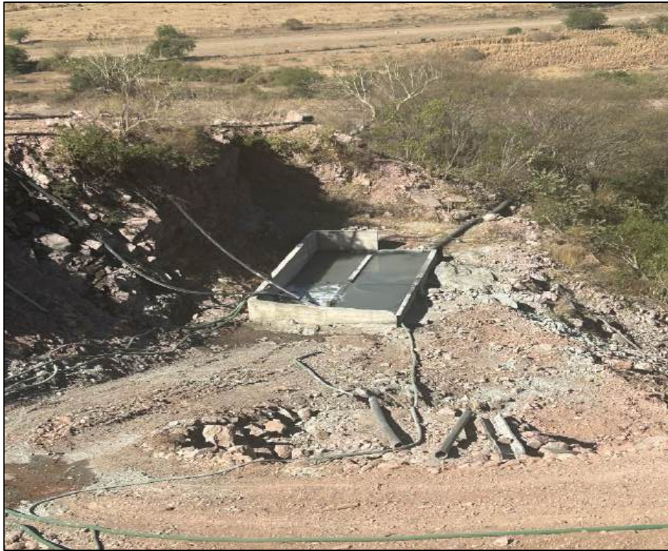
FIGURE 14.15 TAILINGS DECANTED WATER RECOVERY – GRAVITY FLOW TO MILL
