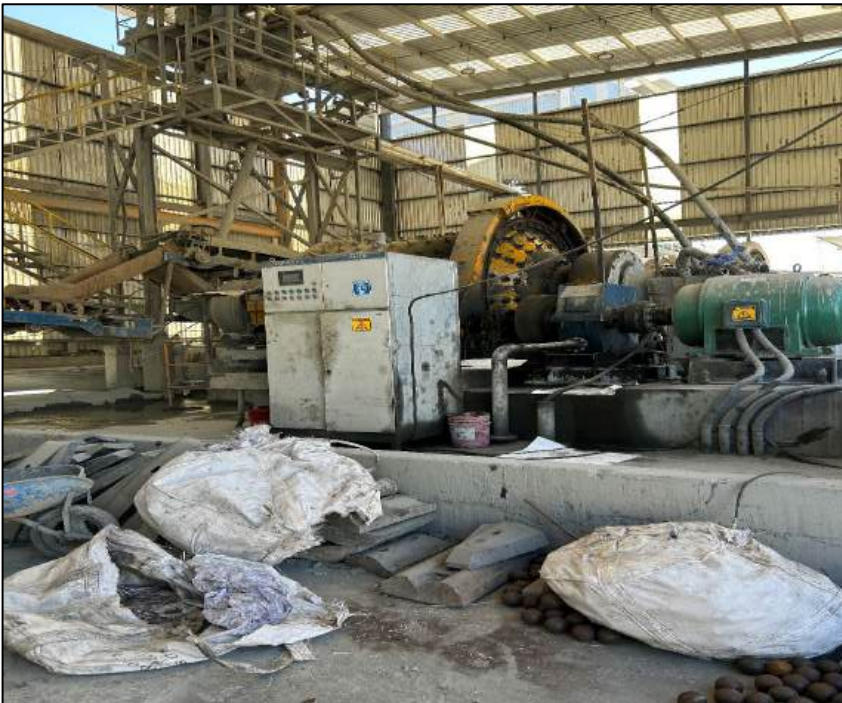
FIGURE 14.5 300 HP PRIMARY BALL MILL CIRCUIT 8 FEET DIAMETER BY 8 FEET LONG
