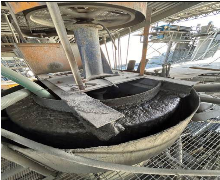
FIGURE 14.7 ROUGHER AND SCAVENGER HYBRID FLOTATION CELLS
