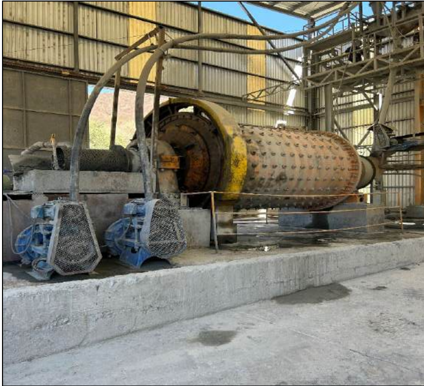
FIGURE 14.4 500 HP PRIMARY BALL MILL CIRCUIT 8 FEET DIAMETER BY 12 FEET LONG
