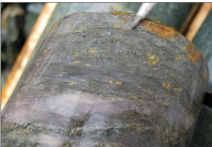
Figure 7.18 Abundant visible gold within a quartz-carbonate-chlorite vein from CCD-11-099, downhole depth 6.0 m
