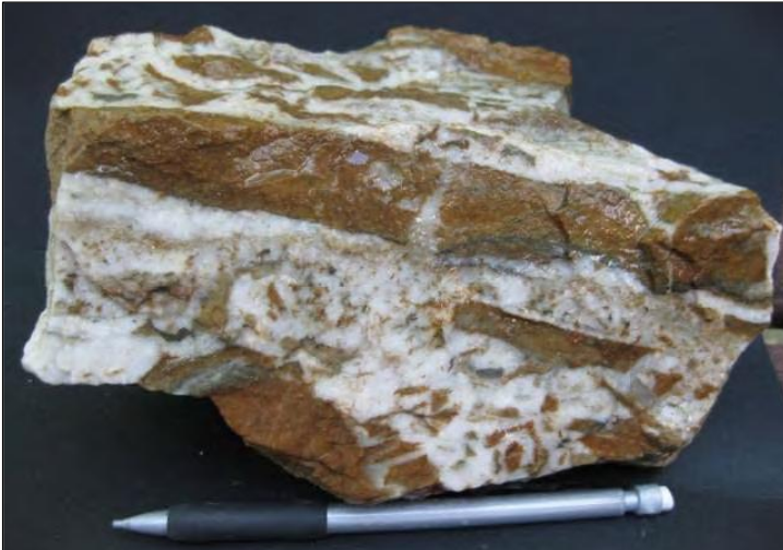
Figure 7.17 Quartz breccia veins with angular altered clasts with disseminated pyrite in a matrix of quartz-pyrite from the Cameron gold deposit stockpile
