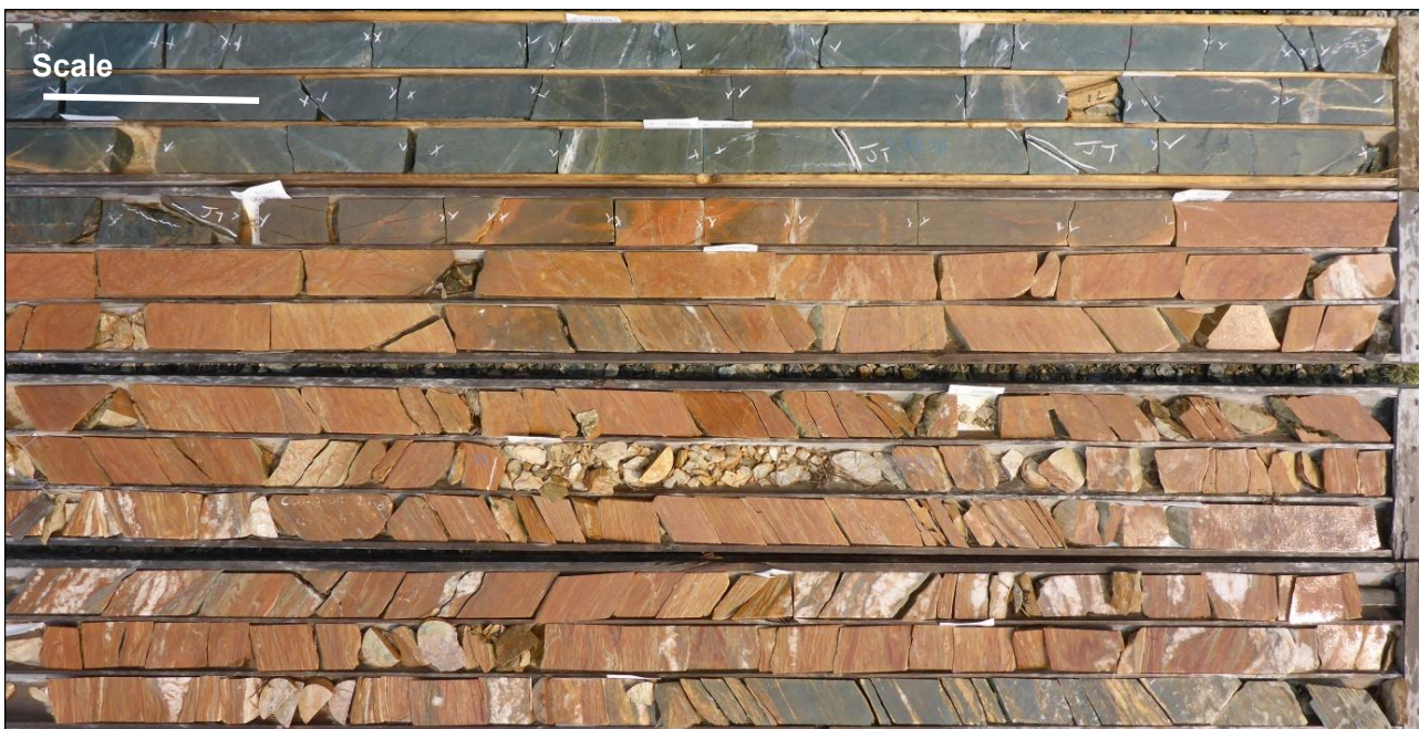
Figure 7.9 Basalt wall rock transition into intensely foliated and ankerite altered mineralized zone with quartz veining in drillhole CCD-10-13
