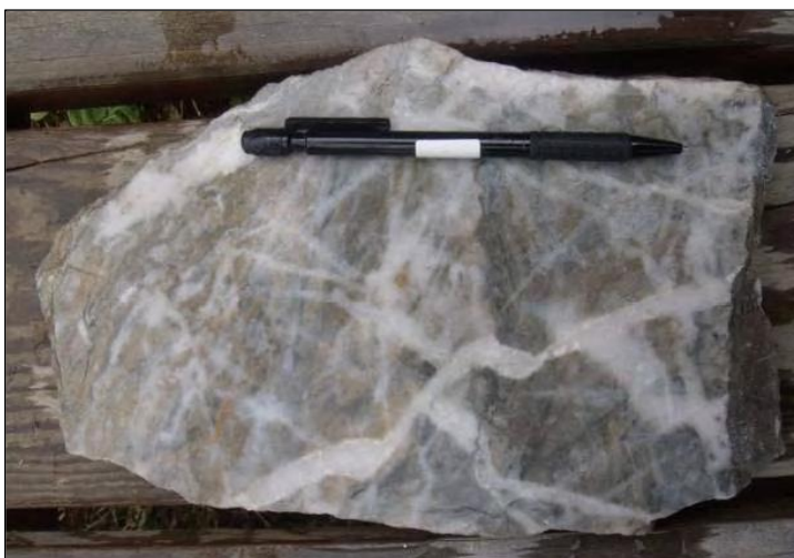
Figure 7.16 Quartz-sulphide stockwork mineralization from the Cameron gold deposit stockpile exhibiting multiple overprinting relationships
