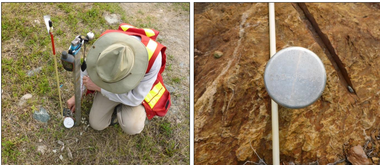
Figure 12.2 GPS and compass checks of Cameron drill collar locations and (left), CCD-11-100 drillhole cap with hole number at deposit outcrop (right)
