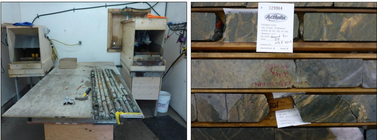
Figure 11.2 Core cutting station and cut core marked up with sampling tickets stapled into the boxes
