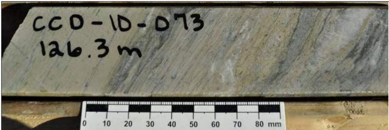
Figure 7.8 Strongly foliated basalt exhibiting typical sericite-iron carbonate-quartz alteration with fine-grained disseminated pyrite from the CLSZ
