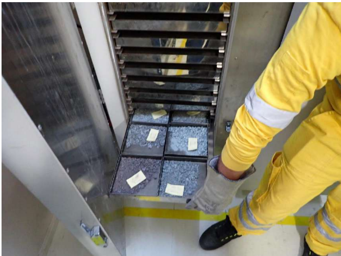
Figure 11.3 Drillhole sample drying oven
