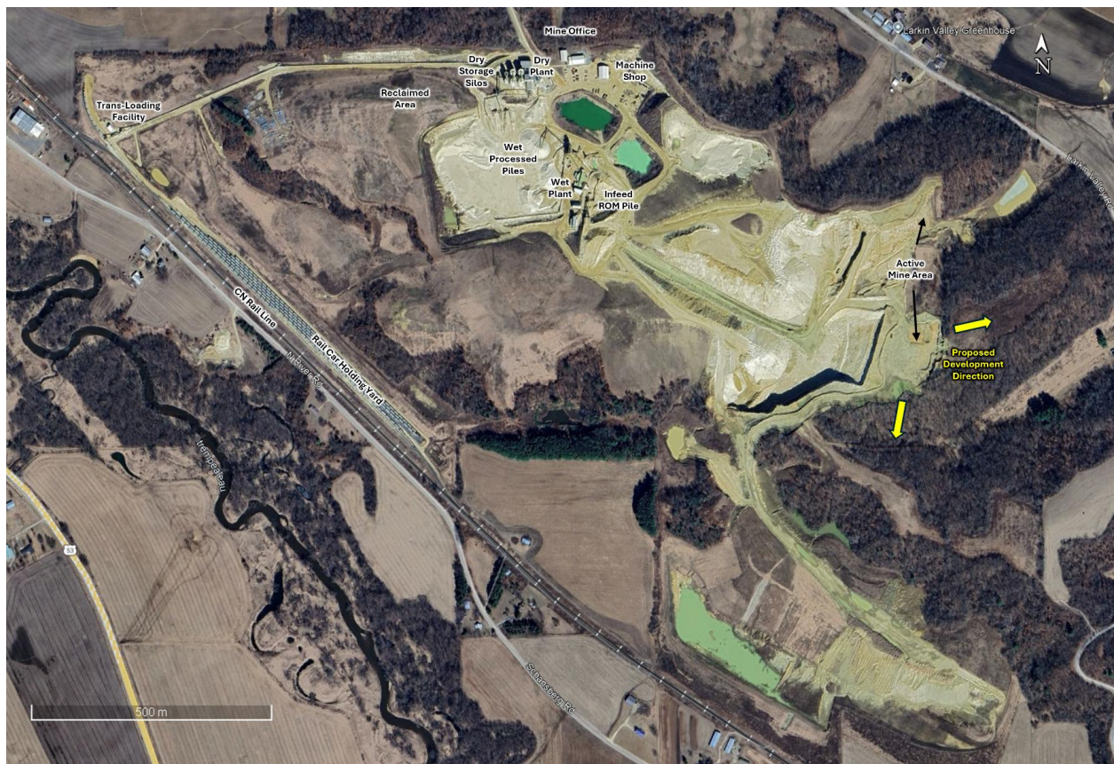
Figure 16.1: Overview of the Significant Infrastructure at the Preston Facility Mine Site. The illustration includes the location of the active mining area, wet and dry processing facilities, product storage areas, waste storage areas, reclamation areas, rail loading terminal, rail car holding yard and proposed direction of future surface mining.
