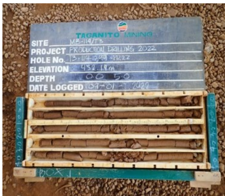
Photo 6. Photograph documentation of a limonite core box in TMC
