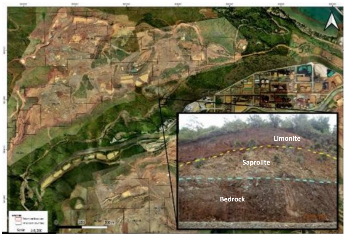
Photo 1. Nickel laterite exposure in TMC and its corresponding profile
