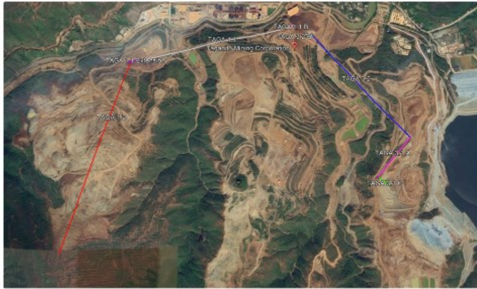
Figure 26. Illustration of the TMC conveyor system (aerial view)
