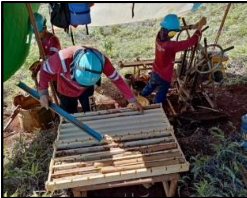
Photo 4. Placing of extracted core sample to the core tray at the foreground. Preparing to resume core drilling in the background.
